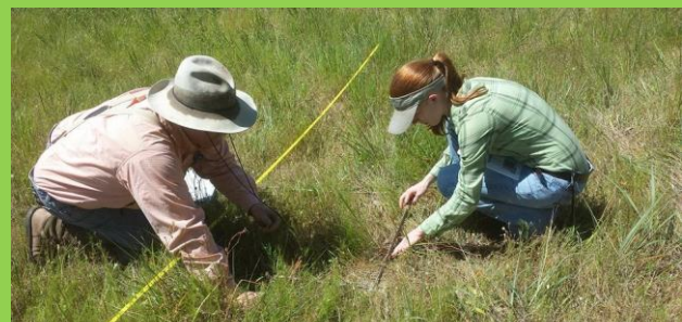
SRM members Erin Wied and Stephen Deiss conducting a vegetative transect for a cooperators in Fayette County, TX. Placing the transect along a permanent line for duplication over time to assess changes helps evaluate the forage base to recommend a correct stocking rate.
